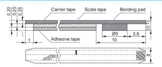
Mechanical isolation of the scale tape from the scale tape carrier; this results in defined thermal behavior.
