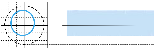
Scanning signal at incorrect mounting conditions before offset and amplitude correction
