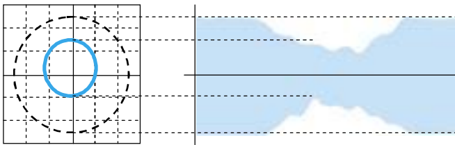
Scanning signal of contaminated scale before offset and amplitude correction
